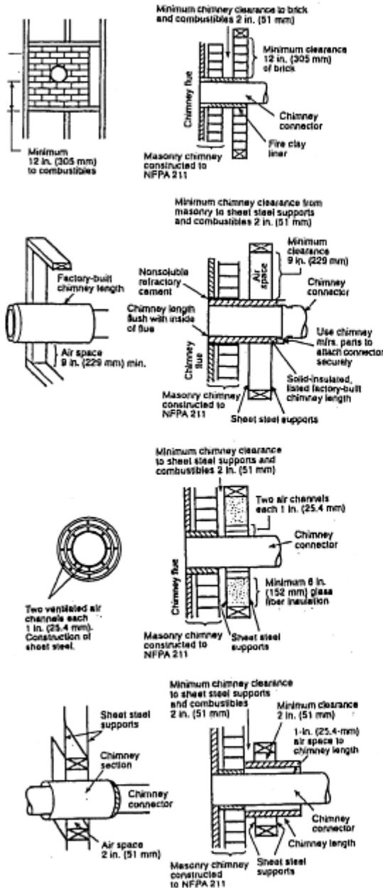
A Minimum 3.5-in thick brick masonry all framed into combustible wall with a minimum of 12-in brick separation from clay liner to combustibles. The fireclay liner shall run from outer surface of brick wall to, but not beyond, the inner surface of chimney flue liner and shall be firmly cemented in place.
