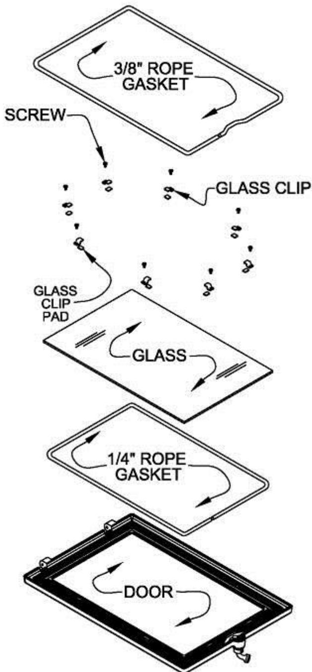
Replace the door glass immediately if broken or chipped. Contact your local dealer for the replacement glass kit PN 90-58405, which is accompanied with instructions and everything needed for the repair. If you replace the glass yourself, wear work gloves and safety glasses.
