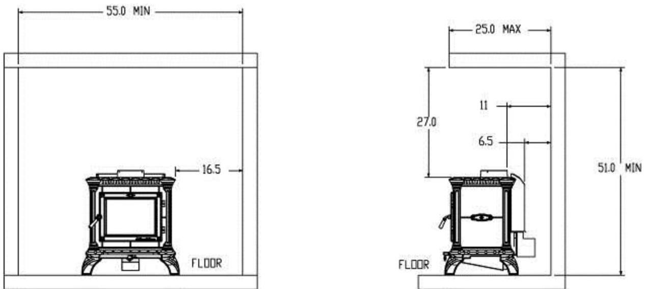
Figure 5: Tribute 8040 Allowable Minimum Alcove Clearances
